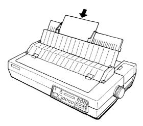
**5.** Press the **LOAD/EJECT** button once to automatically load the paper.
